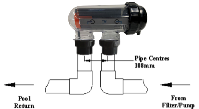
Figure 5. Correct Cell Installation
