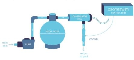
**Note:** Install the Ozone Swim control unit a minimum of 900mm above ground level in an area protected from the elements to eliminate possible damage from severe weather conditions.
