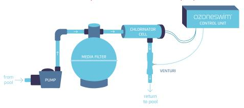
Note: If this system is installed below water level, ensure you have a drain valve fitted to the ozone outlet.
