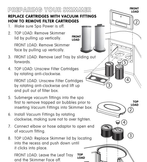
NOTE: Failure to remove air bubbles in the Filters can induce an airlock into the plumbing system, this will cause the pump and heater to operate incorrectly. To ensure there are no airlocks, simply loosen the barrel unions to the pump and heater to release any trapped air and then re-tighten (when conducting this procedure, ensure the Spa Power is OFF).
