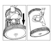
turn, you may have replaced the vanes incorrectly. Place the Shroud back onto the PoolCleaner™ making sure it's on correctly. Drop the three screws into the screw holes and secure.
