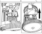
cleaner (the grill). Also make sure that you don't insert the worn side of the vanes into the turbine hub as this would cause them to fall out.
